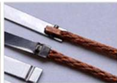
Joining of a harness terminal and a twisted wire (After compacting)
